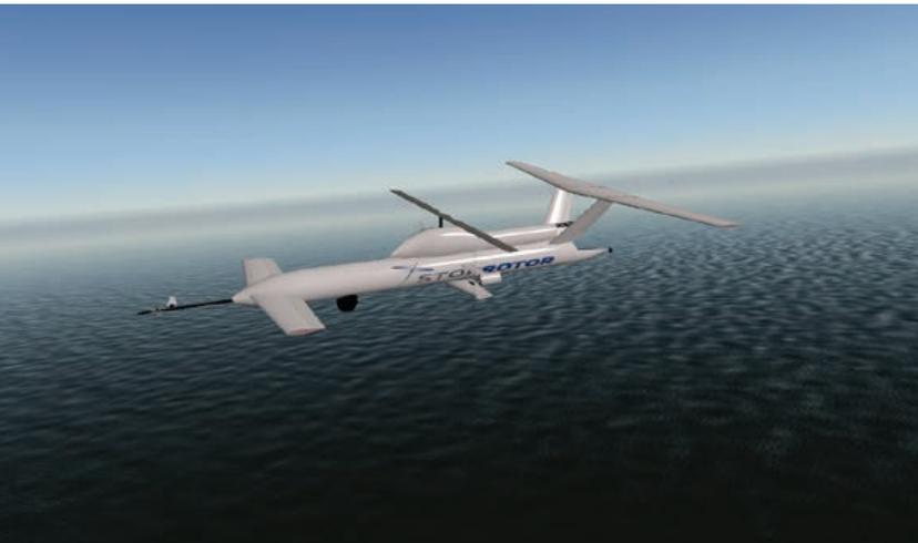
Watkins is the inventor of the **Stoprotor Unmanned Aerial System**, which seeks to combine the best of helicopter and fixed wing aircraft performance.
